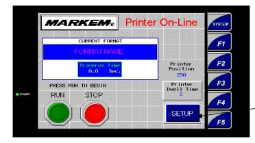
THE PRINTER MUST BE IN THE STOPPED POSITION TO GO TO THE SETUP SCREEN.
