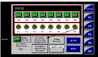
2. PRESS THE "PRINTER VELOCITY SETPOINTS" BUTTON.
