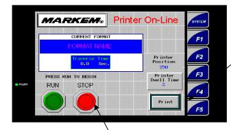
7. PRESS THE "PRINT" BUTTON TO RUN A TEST PRINT.
