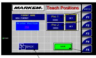
3. PRESS THE "BACK" BUTTON TO EXIT 1. ENTER THE NUMERIC VALUES FOR EACH INDEX BY PRESSING THE POSITION BUTTONS AND KEY THE NUMERIC VALUE FOR EACH POSITION.
