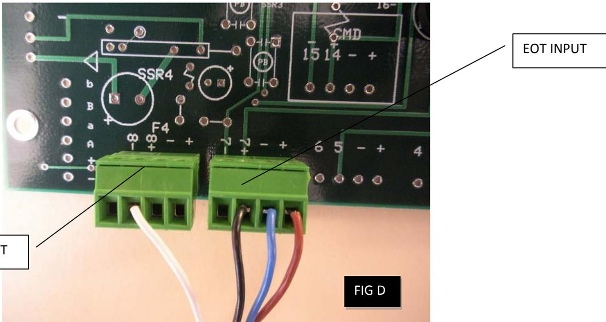
By default; the home sensor wire is connected to input 7+ and the EOT sensor is connected to input 8+ as pictured above (FIG D).
