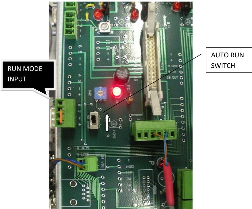
A customer supplied selector switch or relay (maintained) can be wired to the “RUN MODE” input “2
